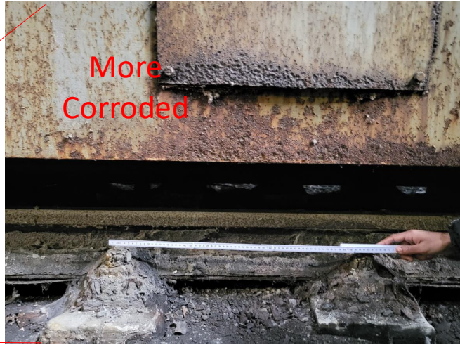
Fig 4 and 5 : The bottom part of towing vehicle - V has more corrosion, photo captured by Sooraj Nair, 2024
